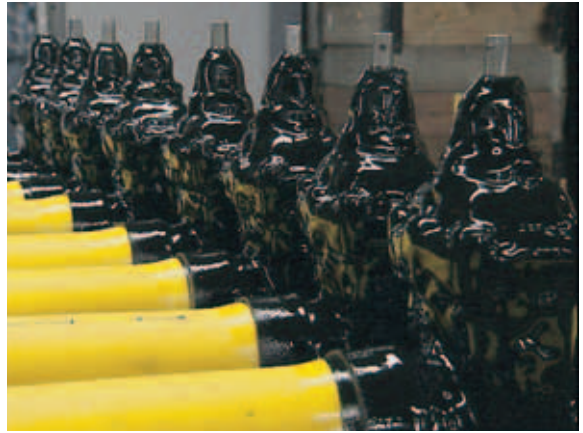
For increased corrosion protection, valves can be coated with polyurethane.
