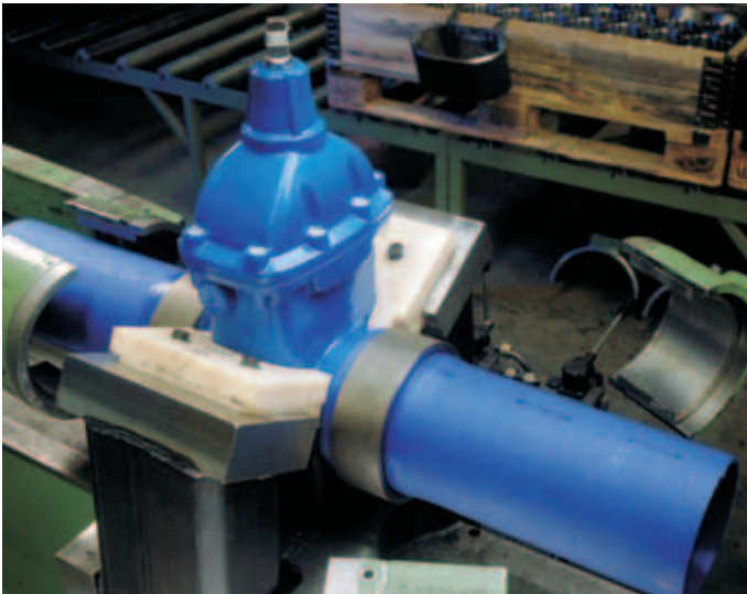
PE-pipes are mounted on the valve (above). Steel sleeves compress the pipe into the valve, providing tensile strength (below).
