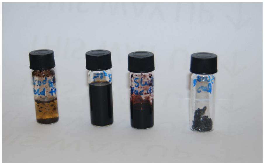
Under the headline “Production of sustainable fuels from sludge and waste”, scientists from i.e. Aarhus and Aalborg universities are working together regarding the so-called HTL-technique (Hydro Thermal Liquefaction); a pressure-cooking based process which converts biomass into raw oil. They each have their pilot facility where different organic materials are tested. The materials count i.e. straw, grass, miscanthus, food waste and wastewater sludge from the treatment plant.
